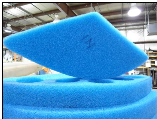
d) First foam baffle piece to be installed
