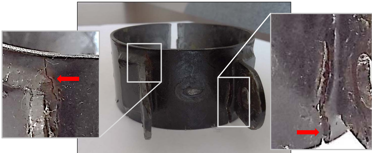
Figure 3. Crack in two locations – each inside the weldment as indicated by the arrows.
