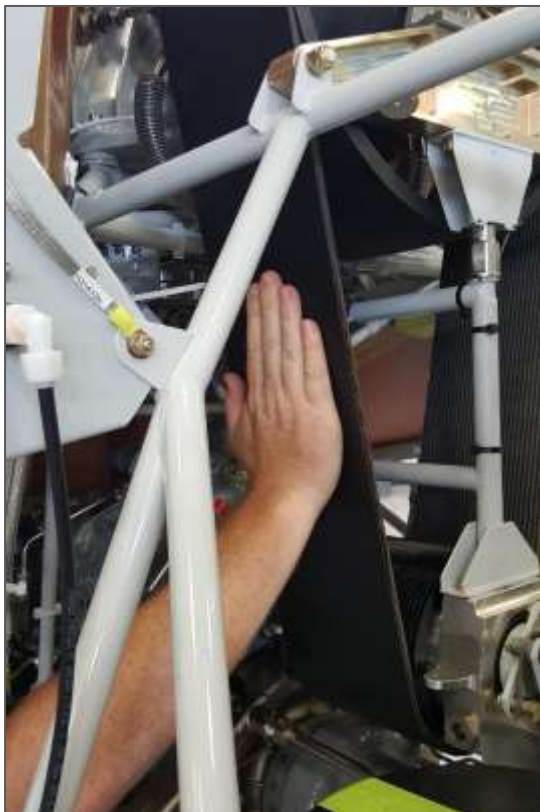
Proper Method – Hand flat against belt surface
