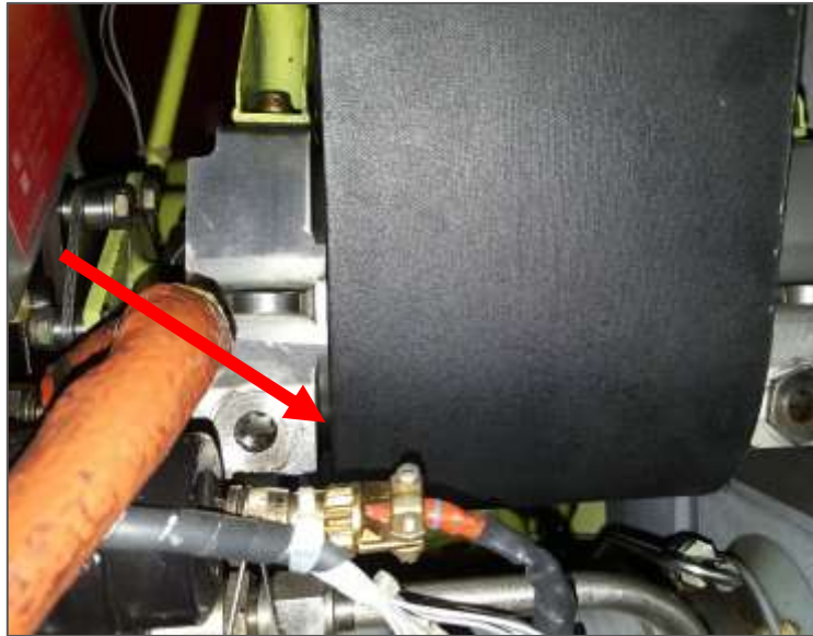
Figure 4a. Inspection point – Lower pulley, forward edge
