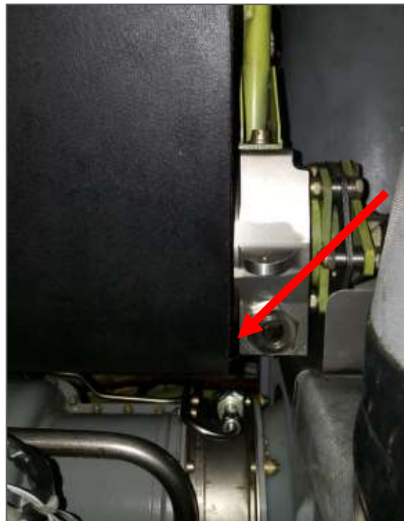
Figure 4b. Inspection point – Lower pulley, aft edge
