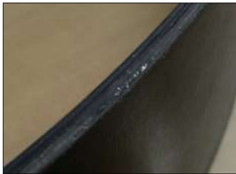
Figure 1. Sealed belt edge
