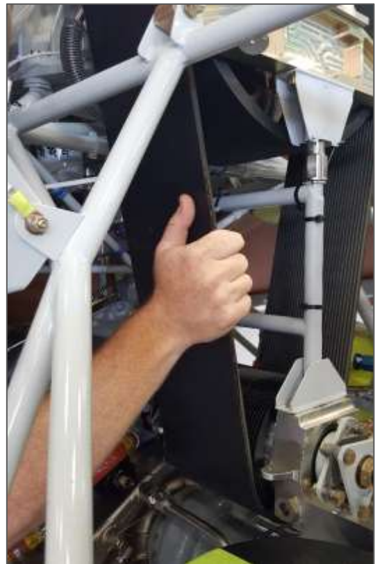
Improper Method – DO NOT grip edge of belt
