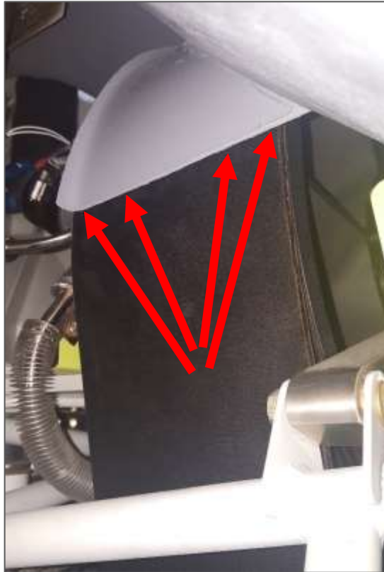
Figure 4e. Inspect upper plenum/air inlet edge for rubber transfer
