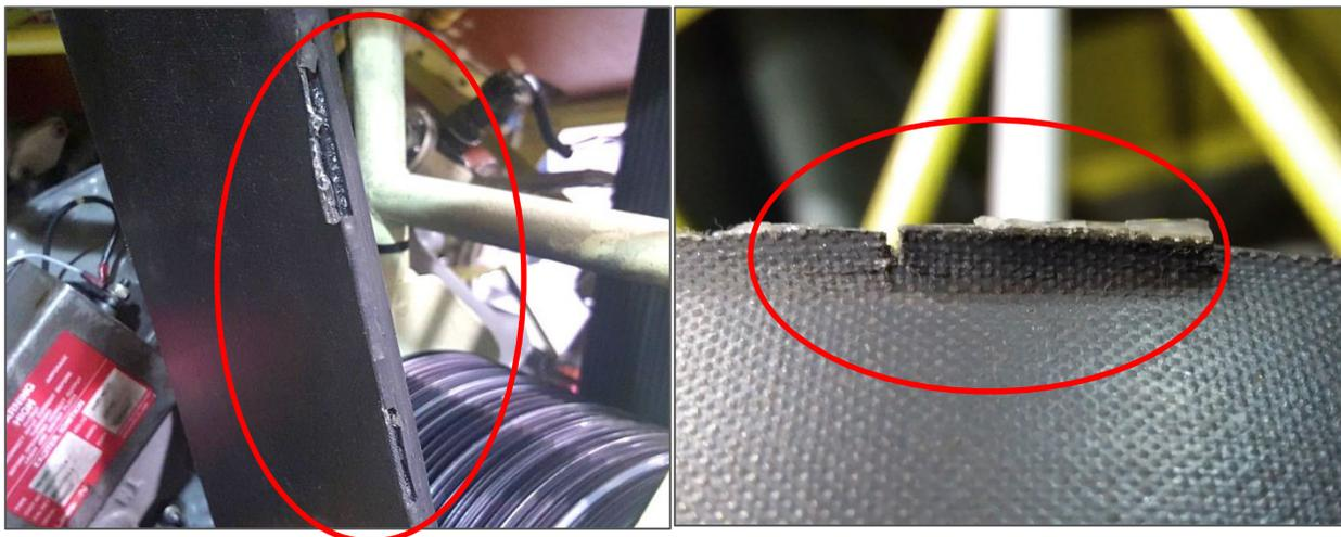
*Figure 2. Deteriorated sealed belt edge (Turbine model drive system shown)*
