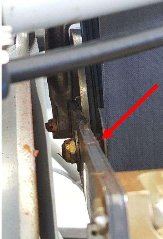
*Figure 4a.* Inspection point – Center pulley, forward edge
