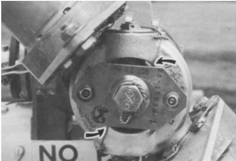
Figure 1: Areas of tail rotor spindle which require particular attention during pre-flight inspection.
