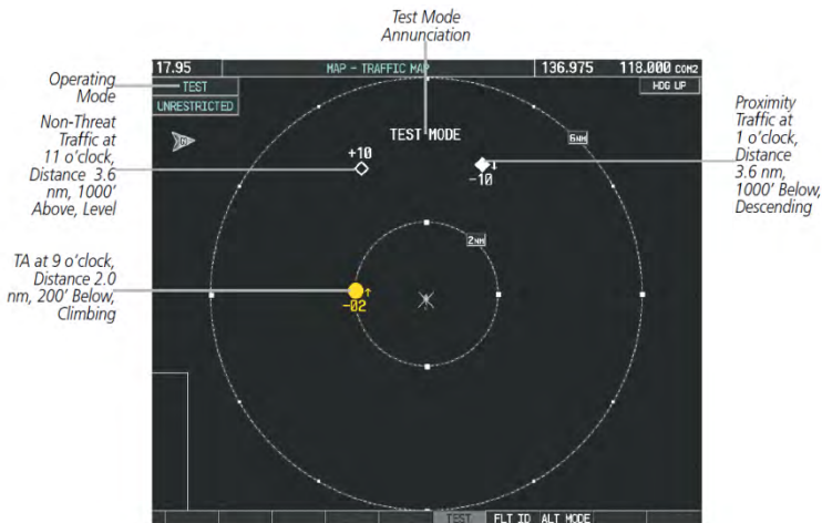
Figure 7-4. System Test in Progress with Test Pattern
