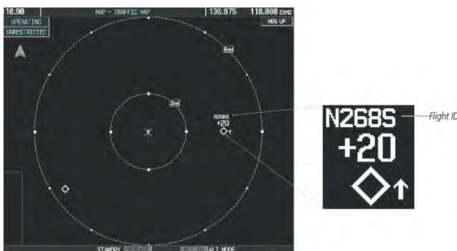
Figure 2-2. Traffic Map Page with Flight IDs Enabled
