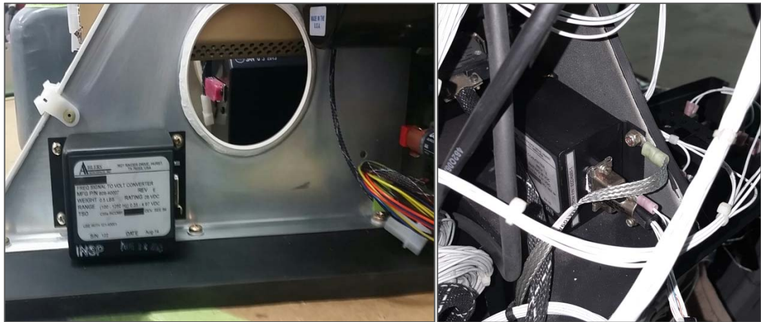
Figure 6. Signal Converter Positioning; Outboard Side of Gusset (left) or Inboard Side of Gusset (right)
