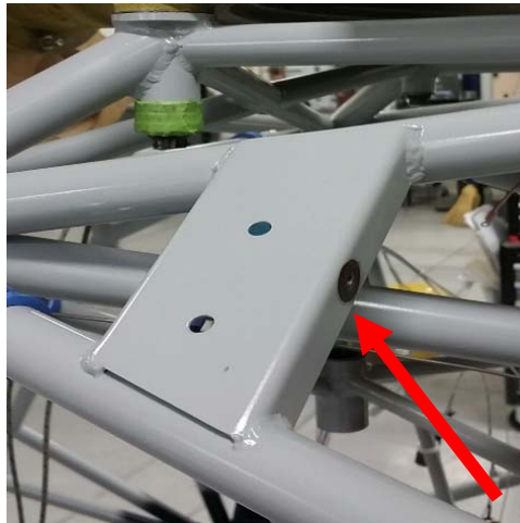
Figure 4. Pylon Gusset Modification (fuel cell structure removed for clarity)
