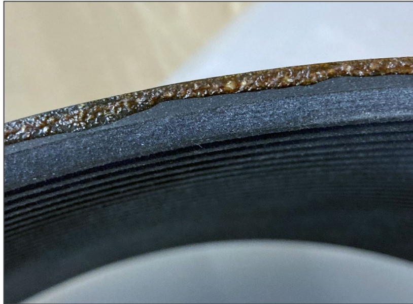
Figure 6. Edge of Belt – Sealed Edge
