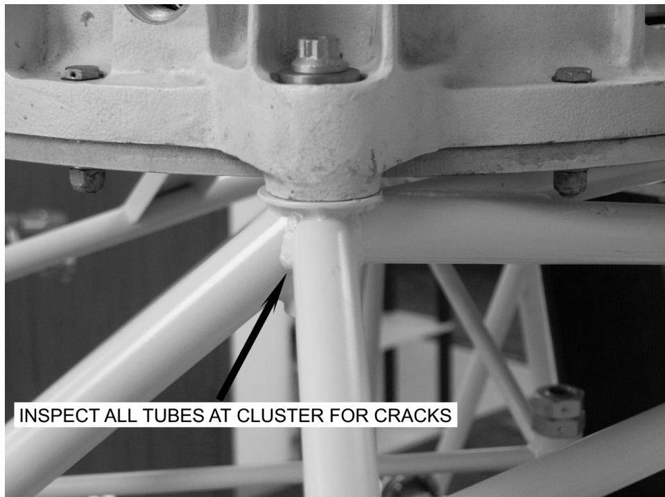
Figure 2. Left, Front Main Rotor Transmission Mount Cluster
