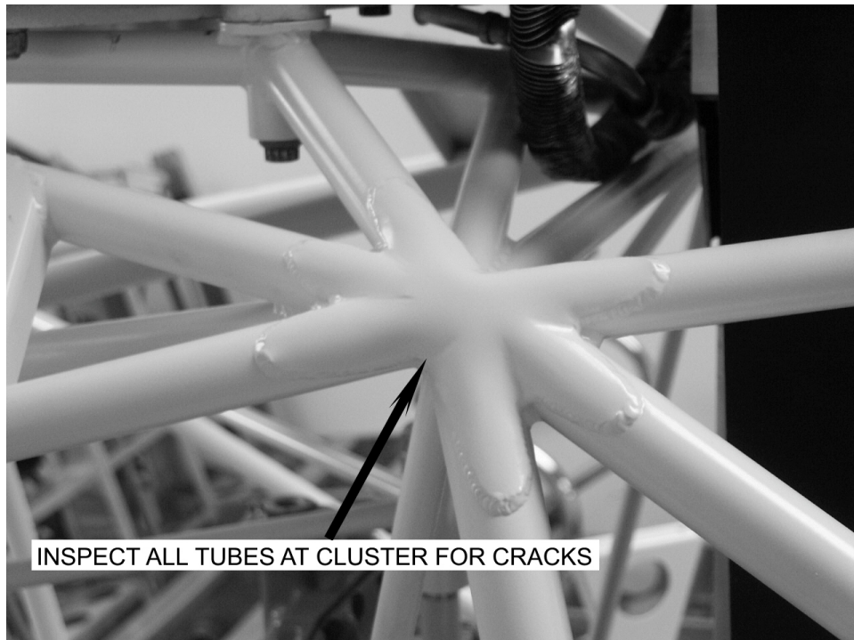
Figure 5. Left, Upper Cluster Located Aft of Transmission Cluster
