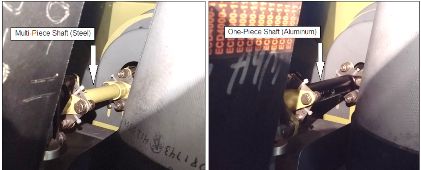
Figure 1. P/N 4129102 shaft as viewed through the left side engine access panel. Multi-piece shaft shown on left; one-piece shaft shown on right.
