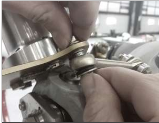
Figure 1. Check for Loose Hardware
