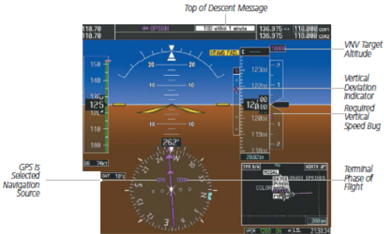
Figure 2-33. Vertical Navigation Indications (PFD)
