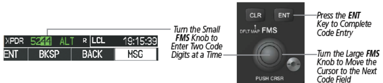
Figure 2-61. Entering a Code with the FMS Knob
