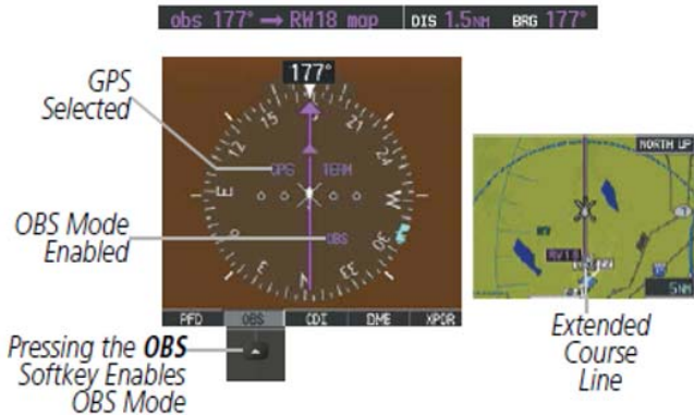
Figure 2-28. Omni-bearing Selector (OBS) Mode Select
