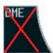
Figure 7-11. DME Power Failure Display
