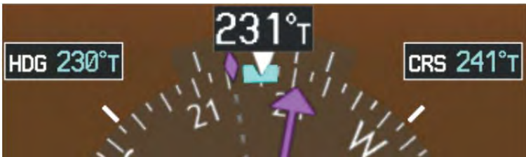
Figure 2-21. Heading and Course Indications (True)
