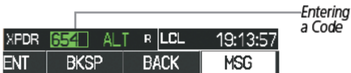
Figure 2-60. Entering a Code
