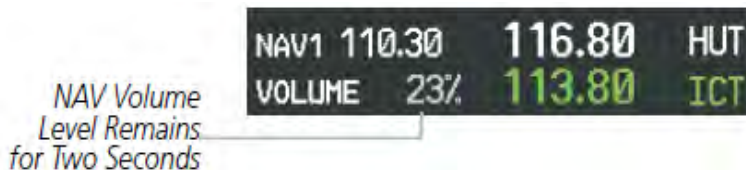
Figure 2-50. NAV Volume Levels
