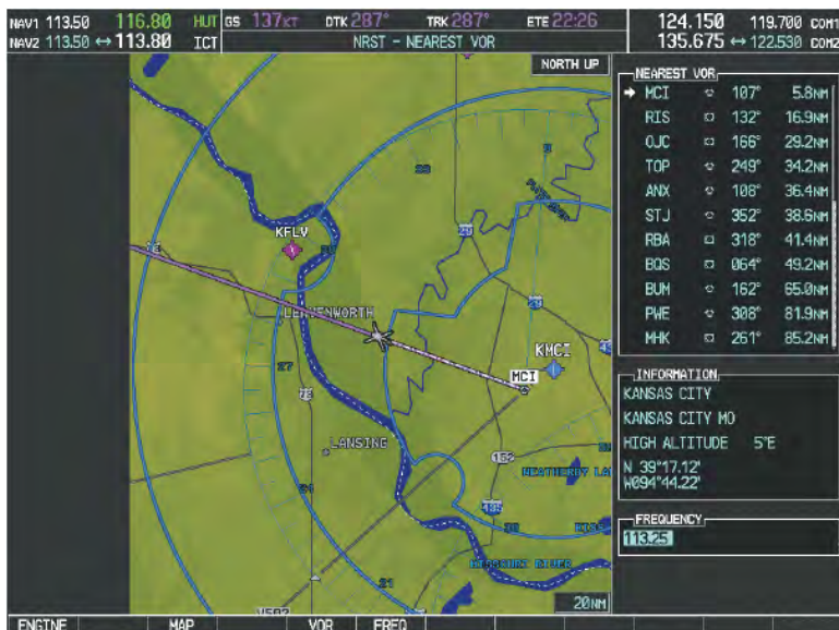
Figure 2-53. Loading the NAV Frequency from the NRST – Nearest VOR Page
