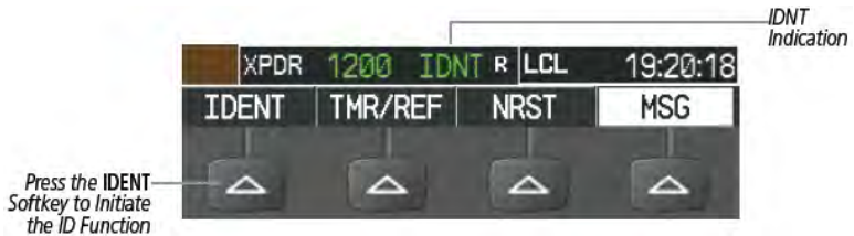
Figure 2-63. IDENT Softkey and Indication
