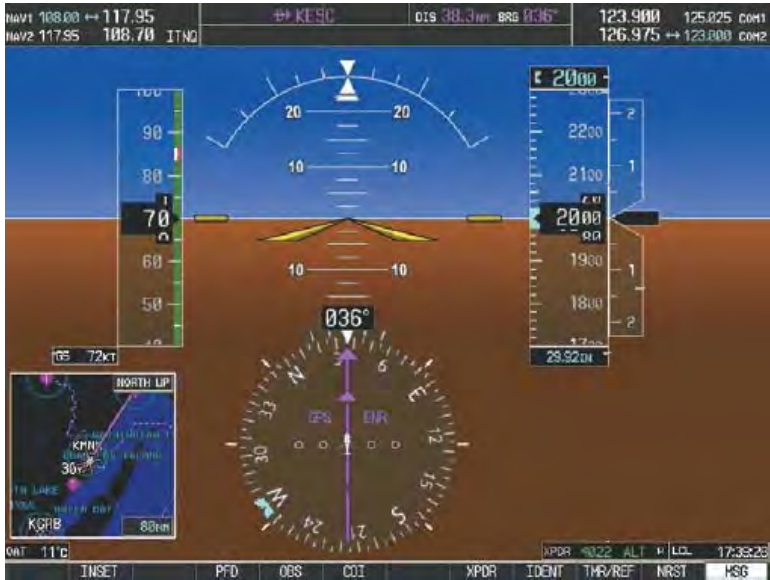
Figure 2-3. PFD Normal Mode
