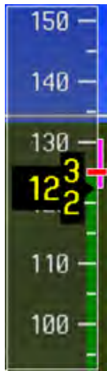
Figure 2-10. Red Pointer at VNE
