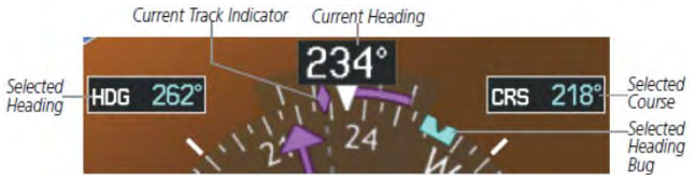
Figure 2-20. Heading and Course Indications
