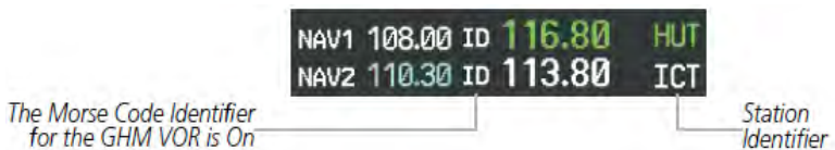
Figure 2-49. NAV Radio ID Indication
