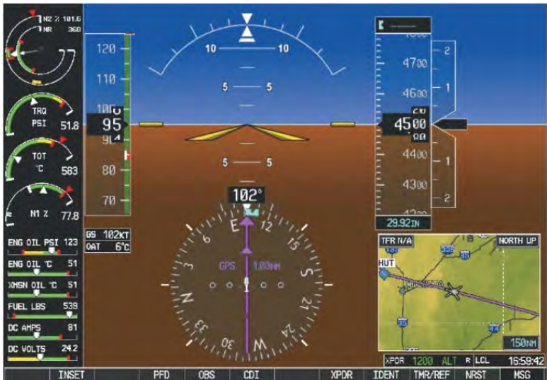
Figure 2-6. MFD Reversionary Mode
