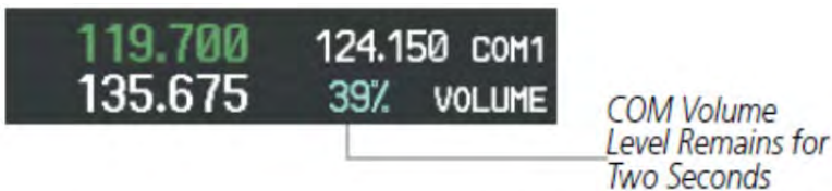
Figure 2-45. COM Volume Level
