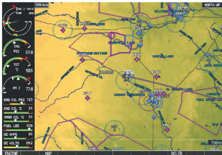
Figure 2-5. MFD Normal Mode
