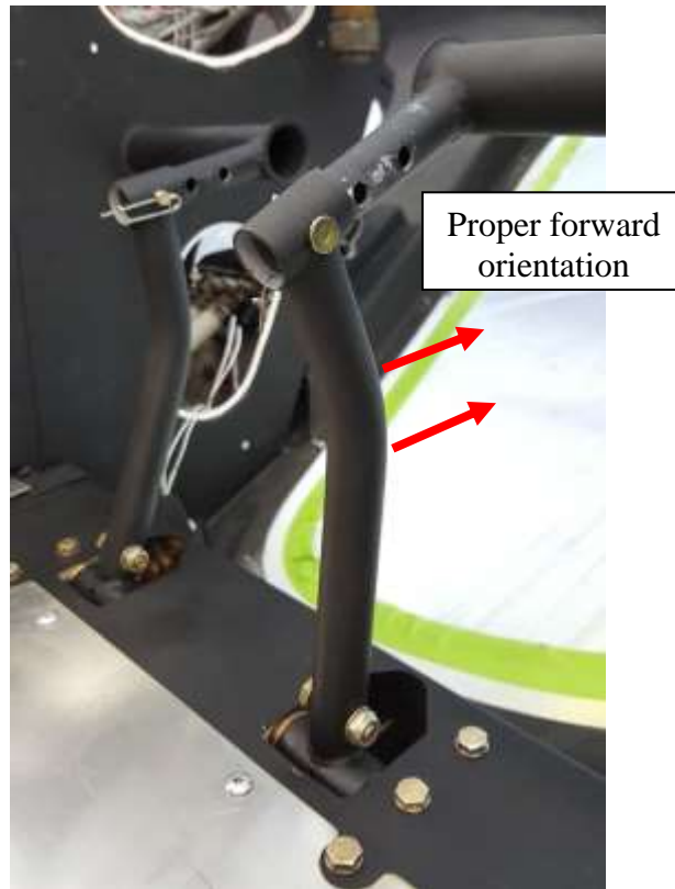
Figure 5. Pedal support leg installation
