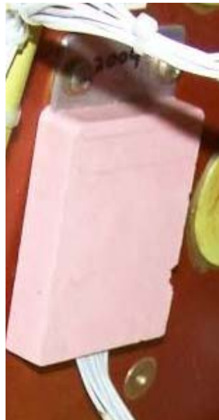
Figure 2: Solid State Trim Switch Unit (NOTE: Color, size, location of the solid state trim switch unit may vary.)
