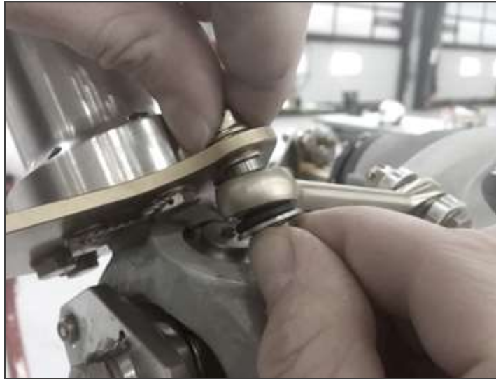
Figure 1. Check for Loose Hardware
