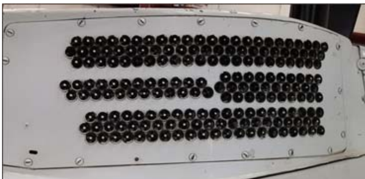
Figure 1. Particle Separator Configurations; ECD4066-1/-2 (a and b), and ECD4066-3/-4 (c)
