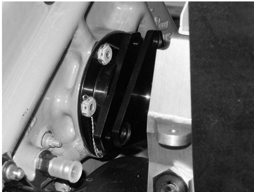
Figure 5 - Engine to Lower Pulley Alignment (Engine Low)
