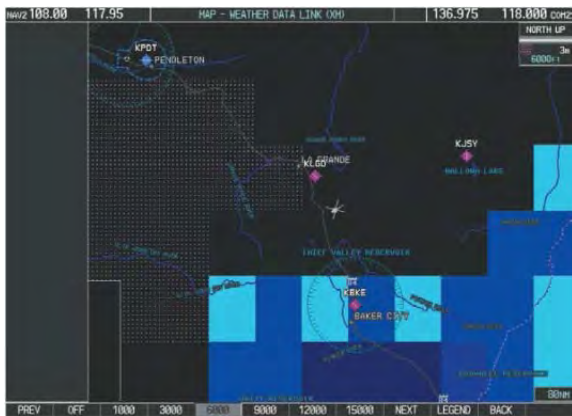
Figure 2-18. Icing Data at 6,000ft.
